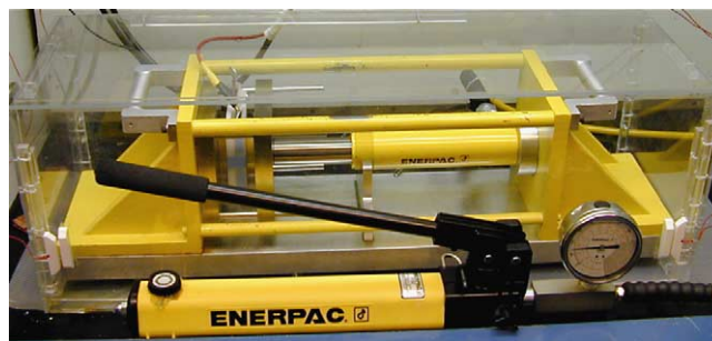
Fig. 16. Apparatus for PPEC with Delrin frame in place. From ref. [38] with permission.
